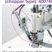
The pneumatic chain-off thread cutter is designed to cut off chain-off thread with a single touch of the knee switch.
