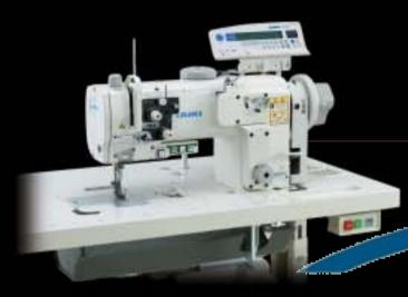
High-speed, 1-needle, Unison-feed, Lockstitch Machine with Vertical-axis Large Hook and **Automatic Thread Trimmer**
